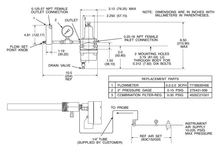
SCHEMATIC HOOKUP FOR REFERENCE AIR SUPPLY ON OXYGEN PROBE.
